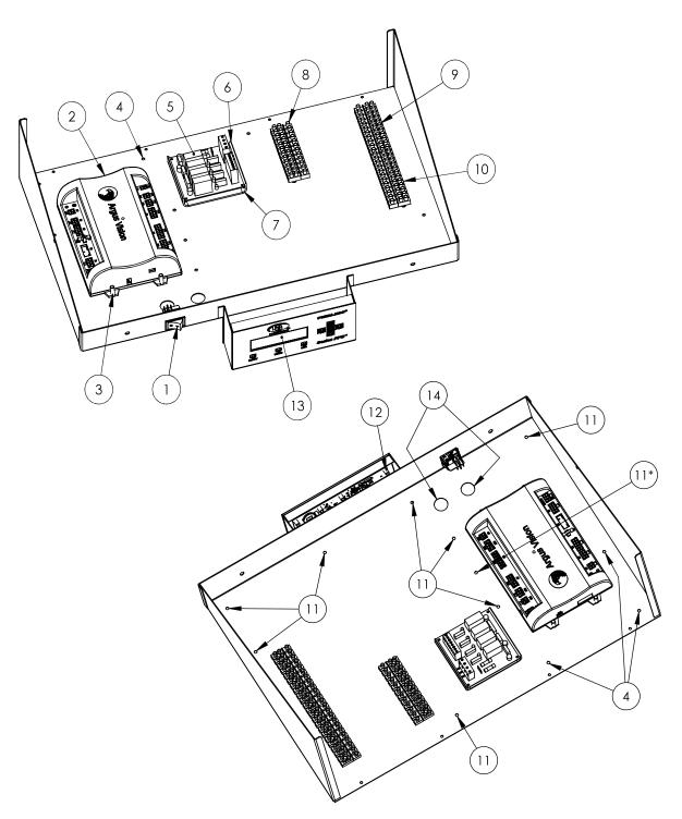
\* THIS WIRE LATCH GATE GOES IN FROM THE BOTTOM SIDE; THE REMAINING LATCHES GO IN FROM THE TOPSIDE.
